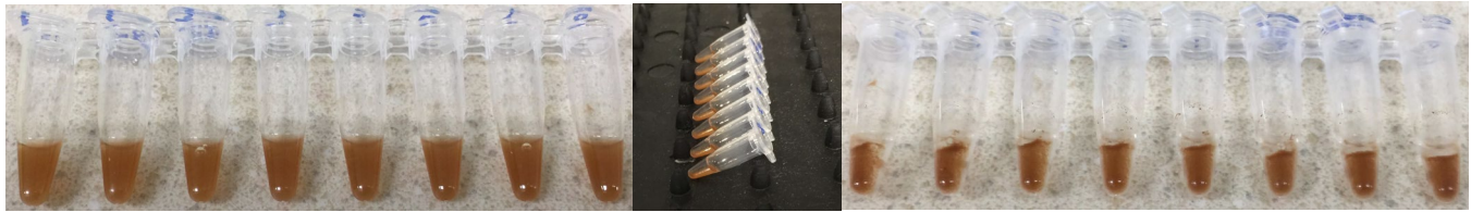
Bead slurry before o/n incubation @ 4°C | nutator o/n | Bead slurry after o/n incubation @ 4°C
