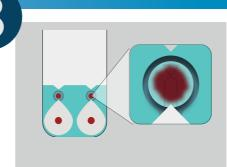
Check the sampling. **Success:** The sample outlet window is filled with blood as shown, ideally in both windows.
