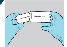
Close the sampling card and attach the sample ID/barcode (g) on the back of the cad and insert the sampling card into the return pouch (f) and close.
