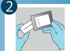
Remove the sampling card (a) from the package. Open the card and put on your table (flat surface). Do not touch the inlets to avoid contamination.
