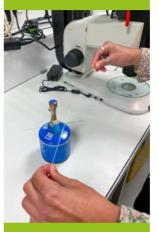
C. The pulled tube is then snapped in the middle, producing two glass transfer pipettes.
