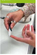
D. The glass transfer pipette is then connected to a Tygon® tube with a blue tip at one end a yellow one at the other end to hold it (then, indeed it is on you to decide!).
